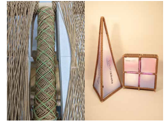
Left: Structurally wound paper yarn element with green sensor yarn Right: Pyramid-shaped display and illuminated counter
