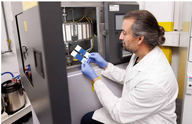
Visual evaluation of fabric samples during color fastness testing against artificial light
