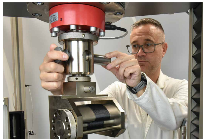
Determination of maximum tensile force and maximum tensile force-elongation on a seat belt
