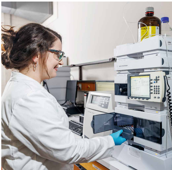
Chromatographs separate substances into their components. In this way, the compositions of mixtures or the molecular weight distribution of polymers can be investigated.
