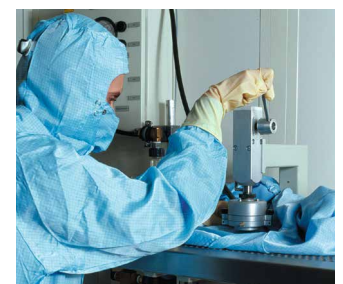
Determination of the particle emission of cleanroom garments using the Suction/Counter method
