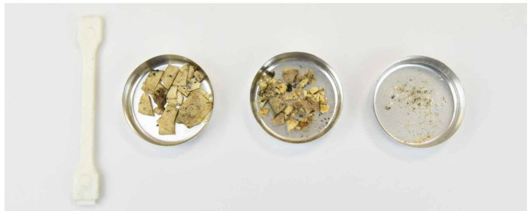
The ARBOBLEND® variant from the company TECNARO shown in the picture is degraded in the routine operation of a biowaste composting plant. (From left to right) before composting, after 2 weeks, after 6 weeks, after 12 weeks.
