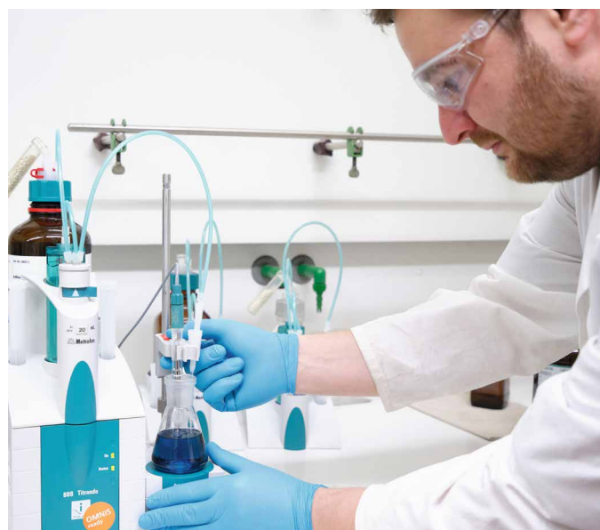
Automated, potentiometric titration is used to determine end groups and thus, for example, the molecular weights of polymers.
