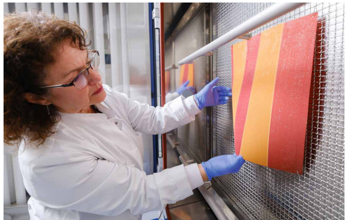
Removal of the awning fabric sample weathered with rain, among other things, for further testing
