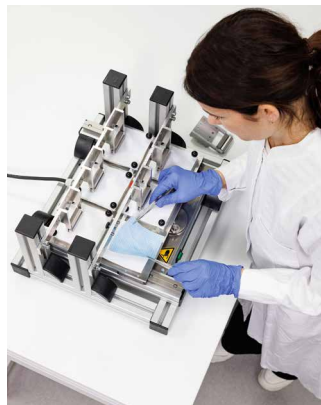
Determination of the bacterial penetration with the ReBa 2 test device
