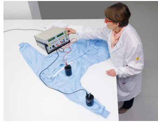
Determination the point-to-point resistance of cleanroom garments for the ESD sector
