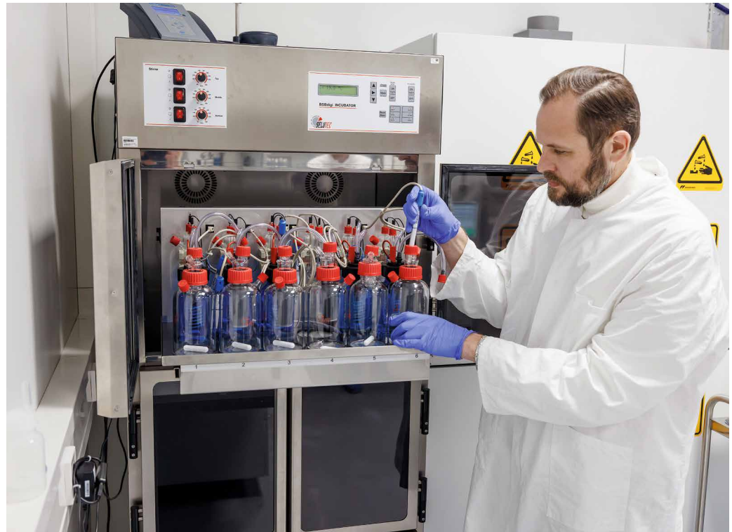
The respirometer examines how a sample degrades. It measures the exchange rate of oxygen and carbon dioxide – in other words, how much is "respired" by the microorganisms. The more they "breathe", the more is biodegraded.
