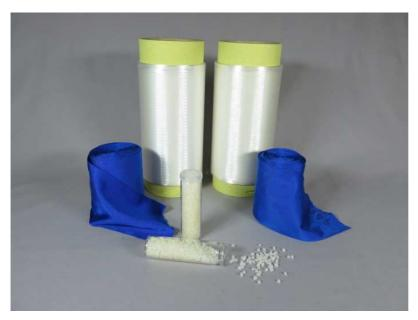
Image: Granules, fibers and dyed fabrics of flame-retardant polyamide
