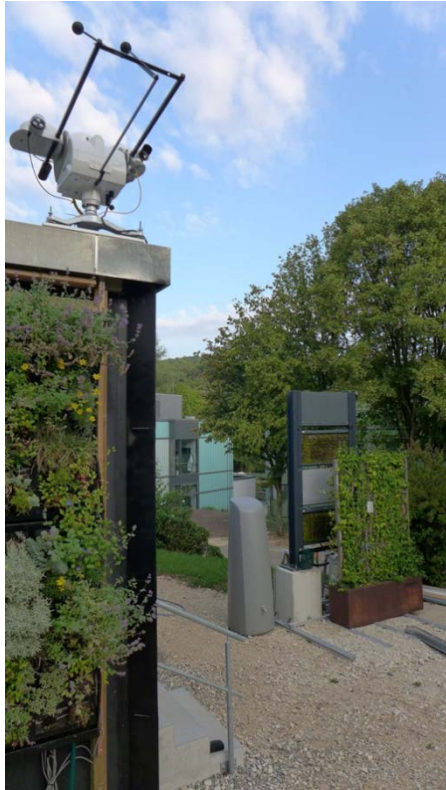
Sun tracker on top of the ForschungskUBUS (left) and demonstration system for a system that reduces particulate matter and provides sound insulation via moss modules and plant-based shading elements. Photo: DITF
