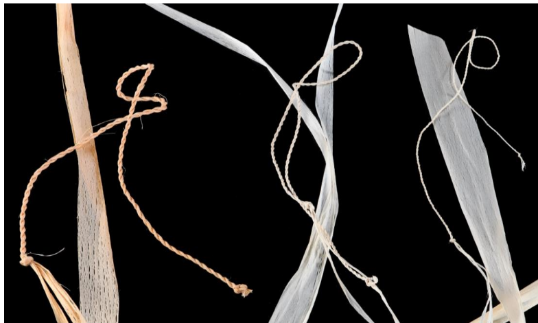
Lime bast: the quality of bast layers and the spliced threads made from them depends on their proximity to the wood of a tree. Spinning proved tedious and difficult, splicing was no problem: Photo: @LAD/YAM
