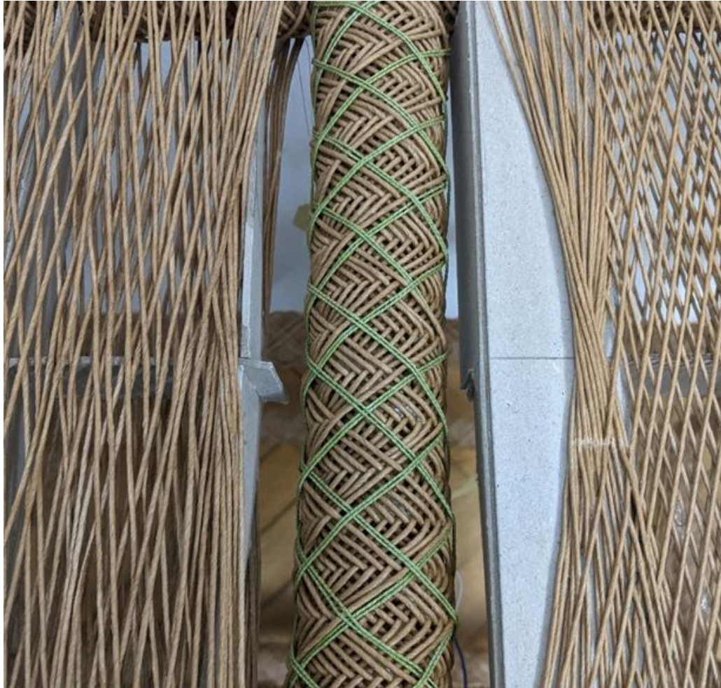
Structurally wound paper yarn element with green sensor yarn. Photo: DITF
