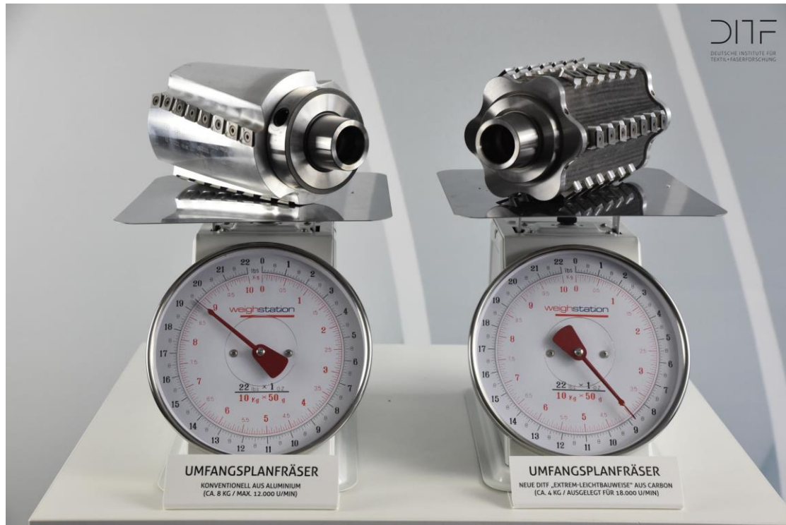
Award-winning planer cutter in extremely lightweight construction. Photo: DITF
