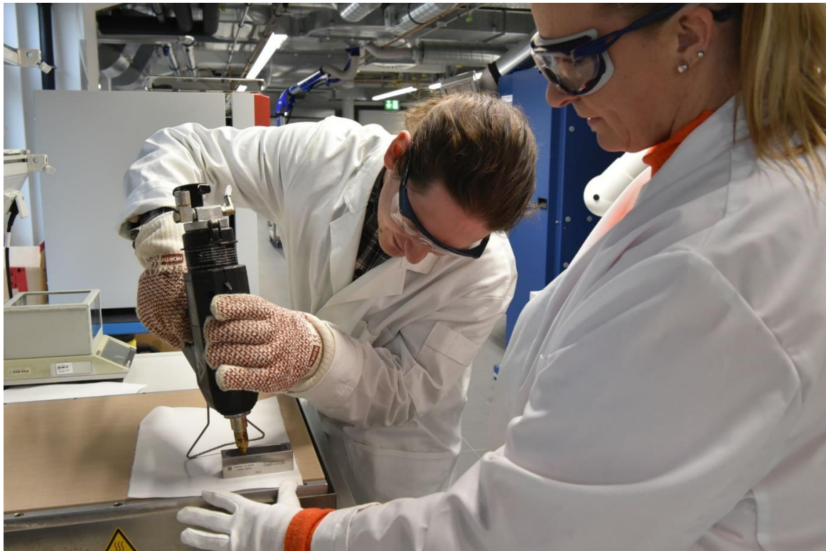
Charging a doctor blade with molten PHA using a hot-melt gun. Photo: DITF
