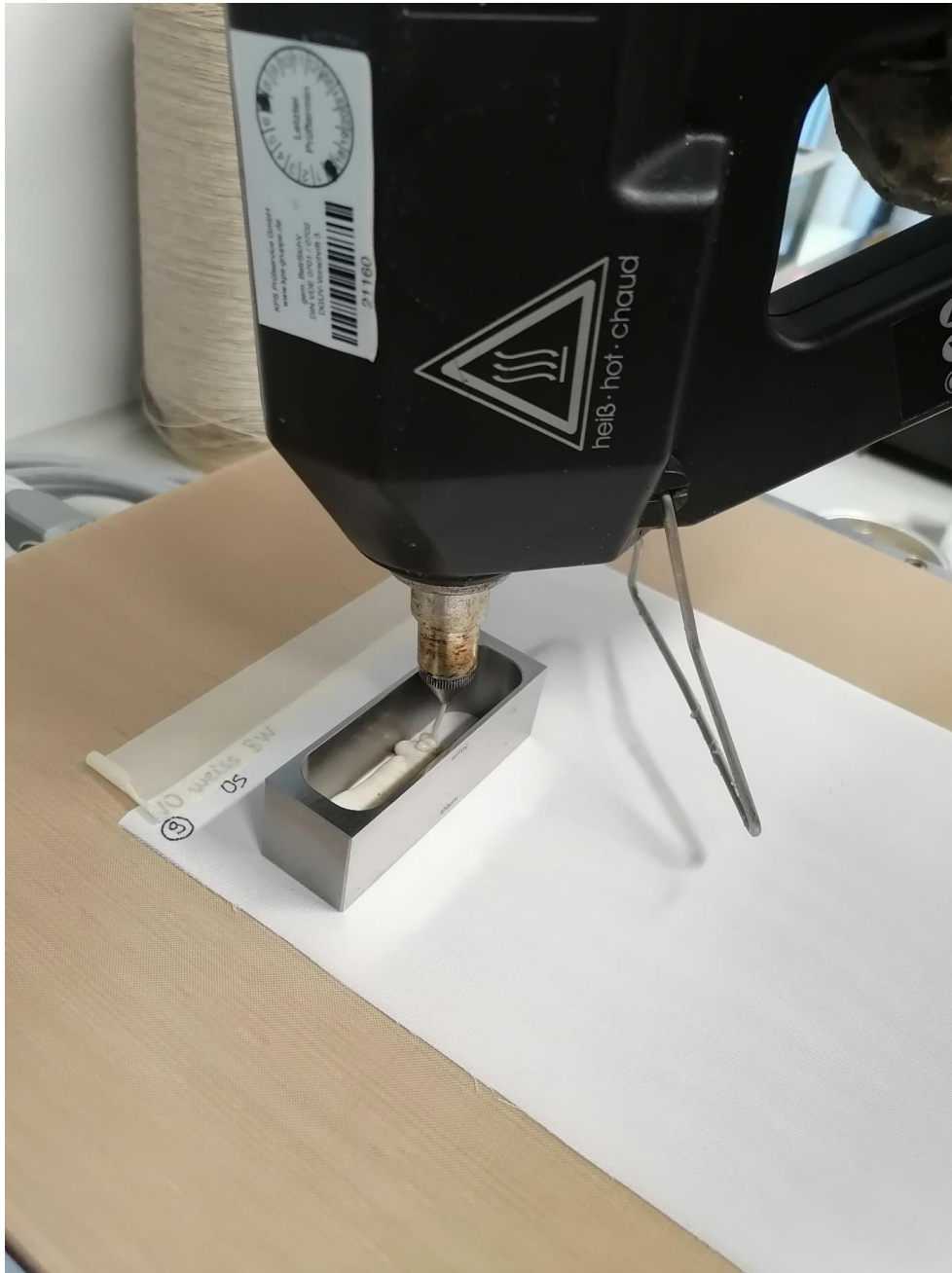
Doctor blade coating of molten PHA on a cotton fabric. Photo: DITF
