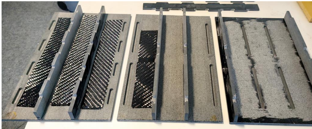
Structure of the wall element. Photo: DITF
