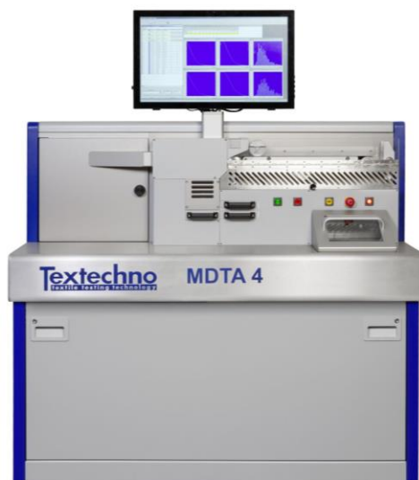
Preparation for the classification of recycled fibers with the MDTA 4 measuring device from Textechno Herbert Stein GmbH & Co. KG. Photo: Textechno
