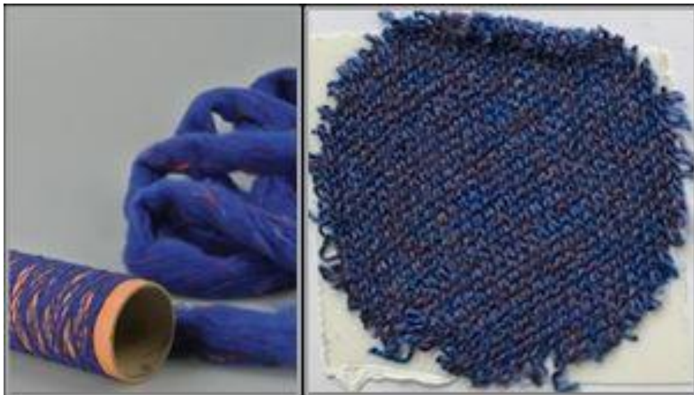
Yarn and knitted fabric made from 100 percent recycled aramid. Photo: DITF
