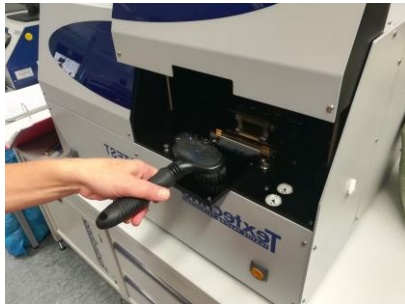
Preparation for the fiber length measurement with the Fibrotest-measuring device (left) Clamped fibers to be inserted into the measuring device (right) Photos: DITF
