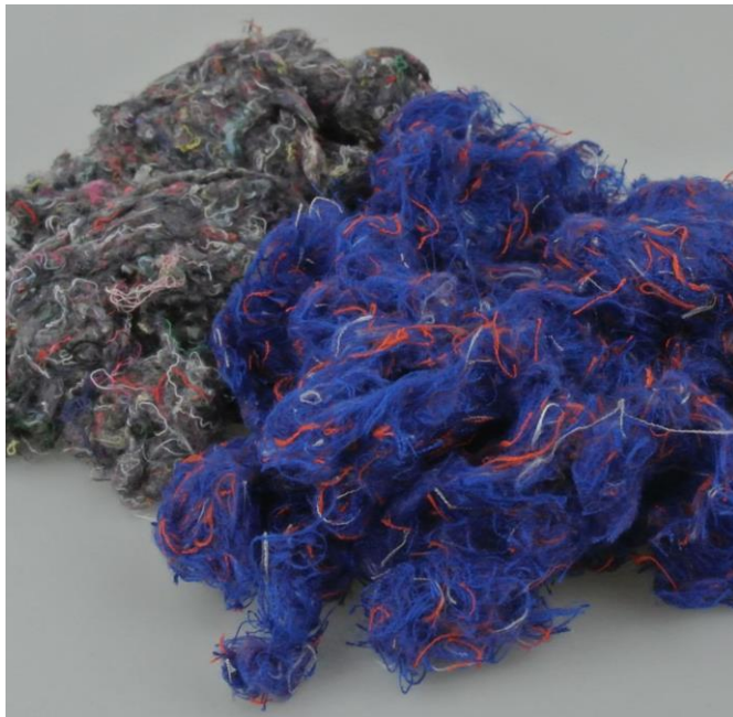
Used textiles after the tearing process. Back: Cotton, front: aramid. Photo: DITF
